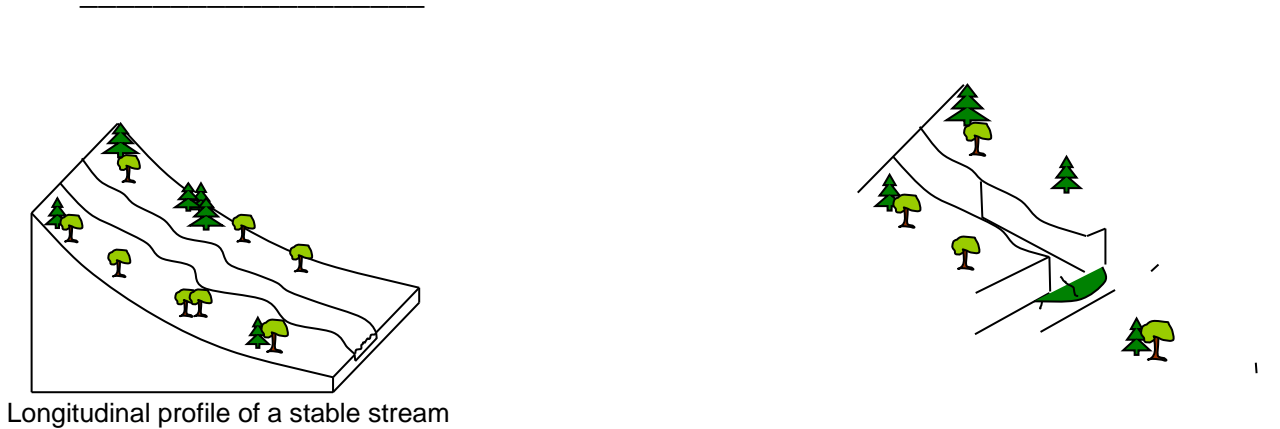
Figure 1: Channel Response to Stream Gravel Removal
